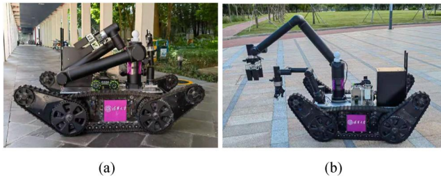
FIGURE 6 Folded and unfolded configurations of the two robotic arms. (a) Folded configuration, and (b) Unfolded configuration.
