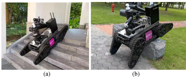
FIGURE 18 HeterBot crossing stairs and high steps. (a) HeterBot crossing stairs. (b) HeterBot crossing high steps.
