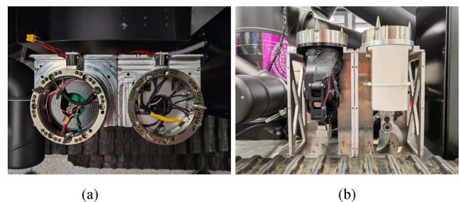
FIGURE 10 Holder of the reconfigurable end effectors. (a) Top view. (b) Side view.
