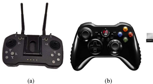
FIGURE 13 The wireless gamepad. (a) Car controller. (b) Arm controller.
